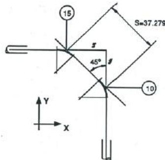
Calculate the  $\Delta$  coordinates to get from the tangent intersection point of the single cut miter bend at node 10 to the single cut miter bend at node 15.
